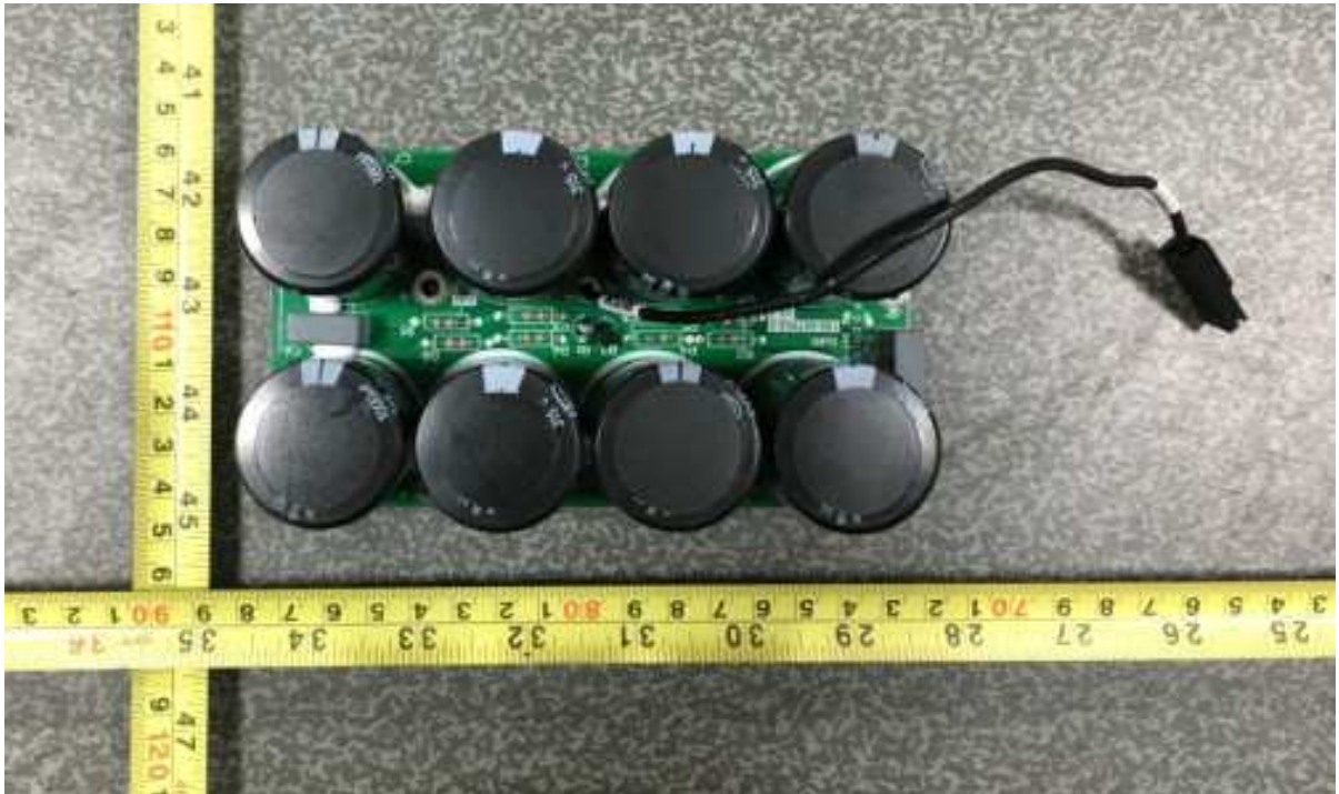
Capacitor board for model HYD 4600-EP, HYD 5000-EP, HYD 5500-EP, HYD 6000-EP
