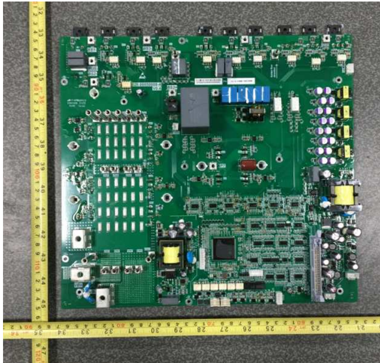
Power board view (Components side)
